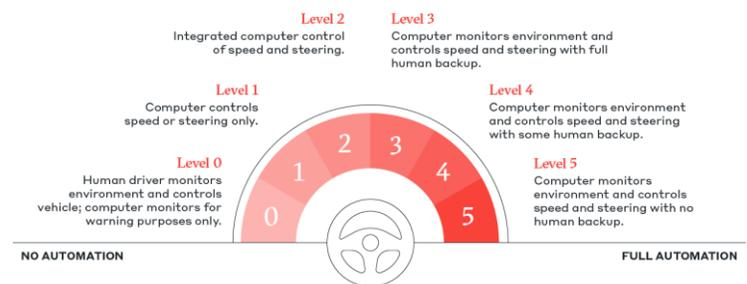
Figure 1 – Adapted from the Society of Automotive Engineers (SAE) standard J3016 levels of driving automation. SAE defines 6 levels of autonomous driving from 0 to 5 based on the human intervention required for the ride. The higher the level of automation, the more information the vehicle uses about the driving environment to automate driving tasks. For SAE levels 1-3, the human driver is required to perform some or all of the driving task(s).<sup>1</sup>
