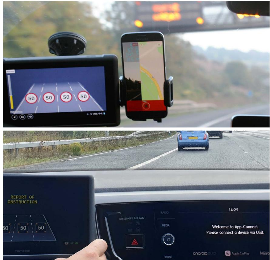
Figure 4 - A2M2 Connected Vehicle Corridor trial of in-vehicle 'virtual gantries'
