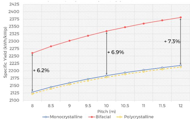
Figure 1 - Relationship between pitch and specific yield for identically modelled monofacial and bifacial indicative 25MW sites.
