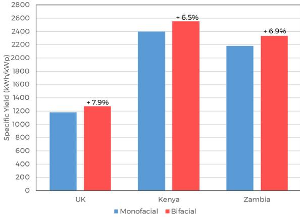
**Figure 2 - Comparison of specific yield between monofacial monocrystalline & polycrystalline and bifacial**
