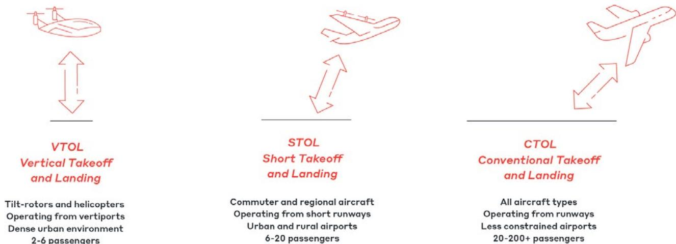
Figure 1 - electric and hybrid aircraft – from VTOL to STOL: Mission requirements drive aircraft performance.
