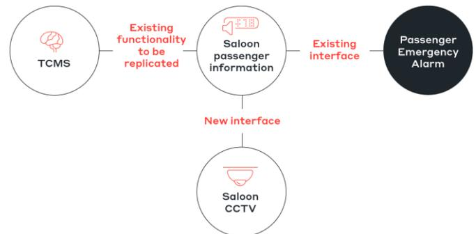
A snapshot of the interfaces that required management are shown in the following context diagram.
