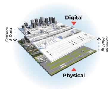
Figure 2 - Elements of a digital twin - A digital twin is a virtual replica of an asset that incorporates associated real-time data during operation of that asset. It provides an immersive and integrated visualization of previously siloed information and enables use of modern digital analysis techniques, such as condition-based monitoring and predictive analysis, to plan for the continued functioning of infrastructure.
