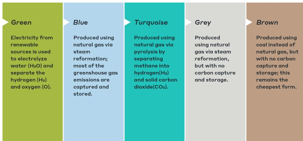
Figure 3 – Five Shades of Hydrogen – Source: Control Risks<sup>7</sup>
