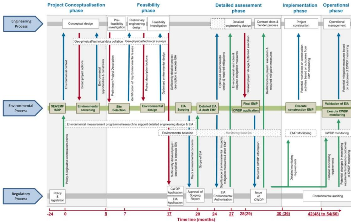
Project lifecycle associated with the development of intake and outfall infrastructure, highlighting the interdependency of engineering, environmental and regulatory processes and associated information flow requirements (after van Ballegooyen et al., 2016).
