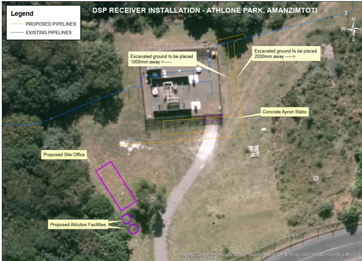
Sasol PRS and the proposed structures and pipeline associated with the Receiver Station (to be constructed on apron slabs)
