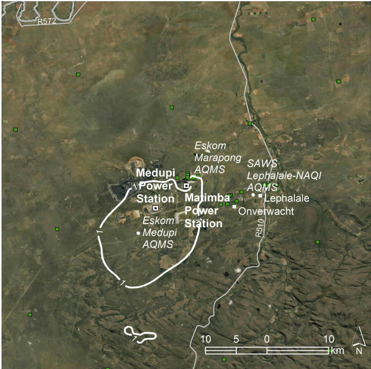
Figure 7-25: Predicted annual average NO 2 concentrations in µg/m 3 resulting from emissions from Matimba: Scenario D (MES) (NAAQS Limit is 40 µg/m 3 )
