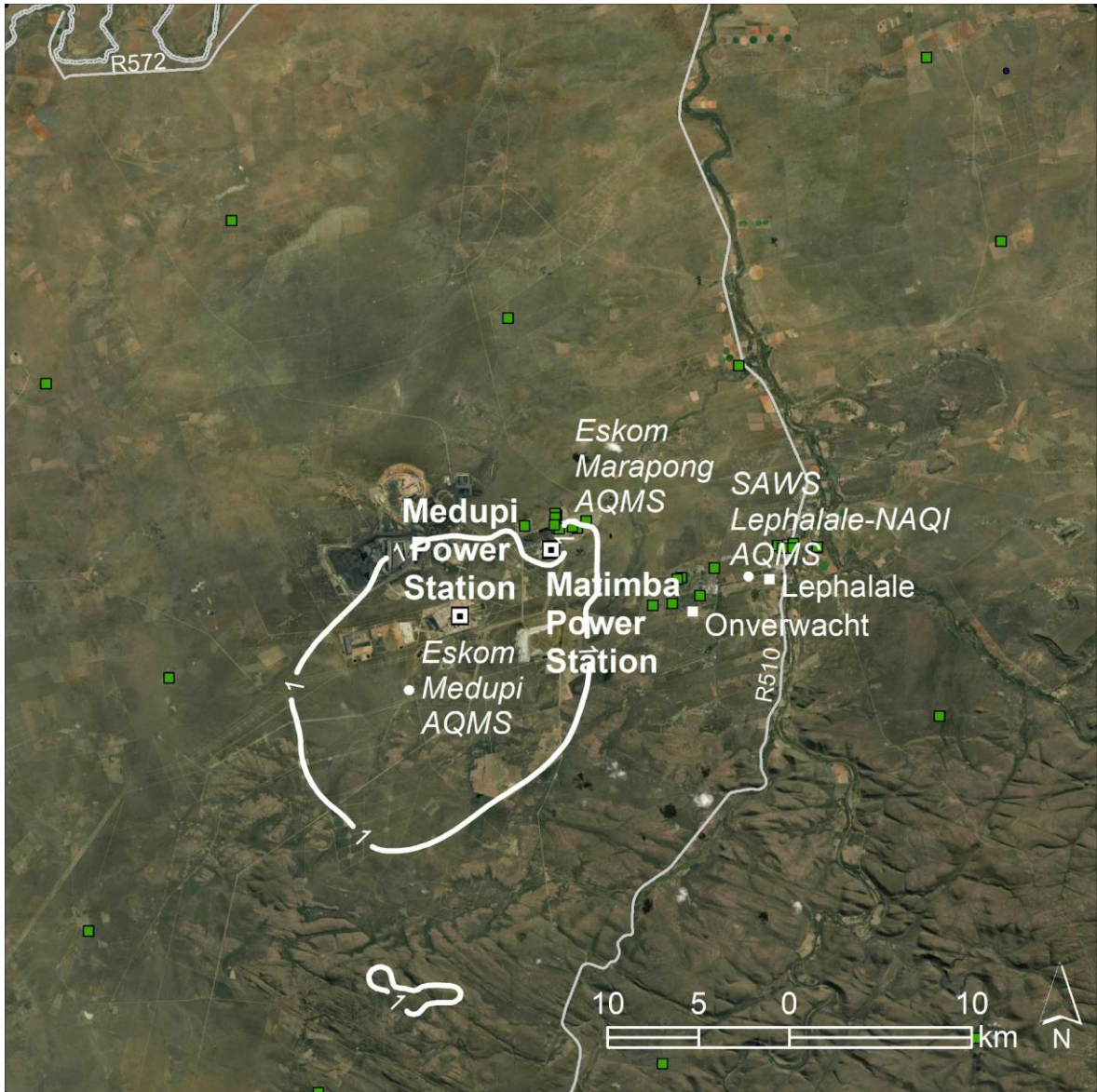
Figure 7-23: Predicted annual average NO 2 concentrations in µg/m 3 resulting from emissions from Matimba: Scenario C (2036) (NAAQS Limit is 40 µg/m 3 )
