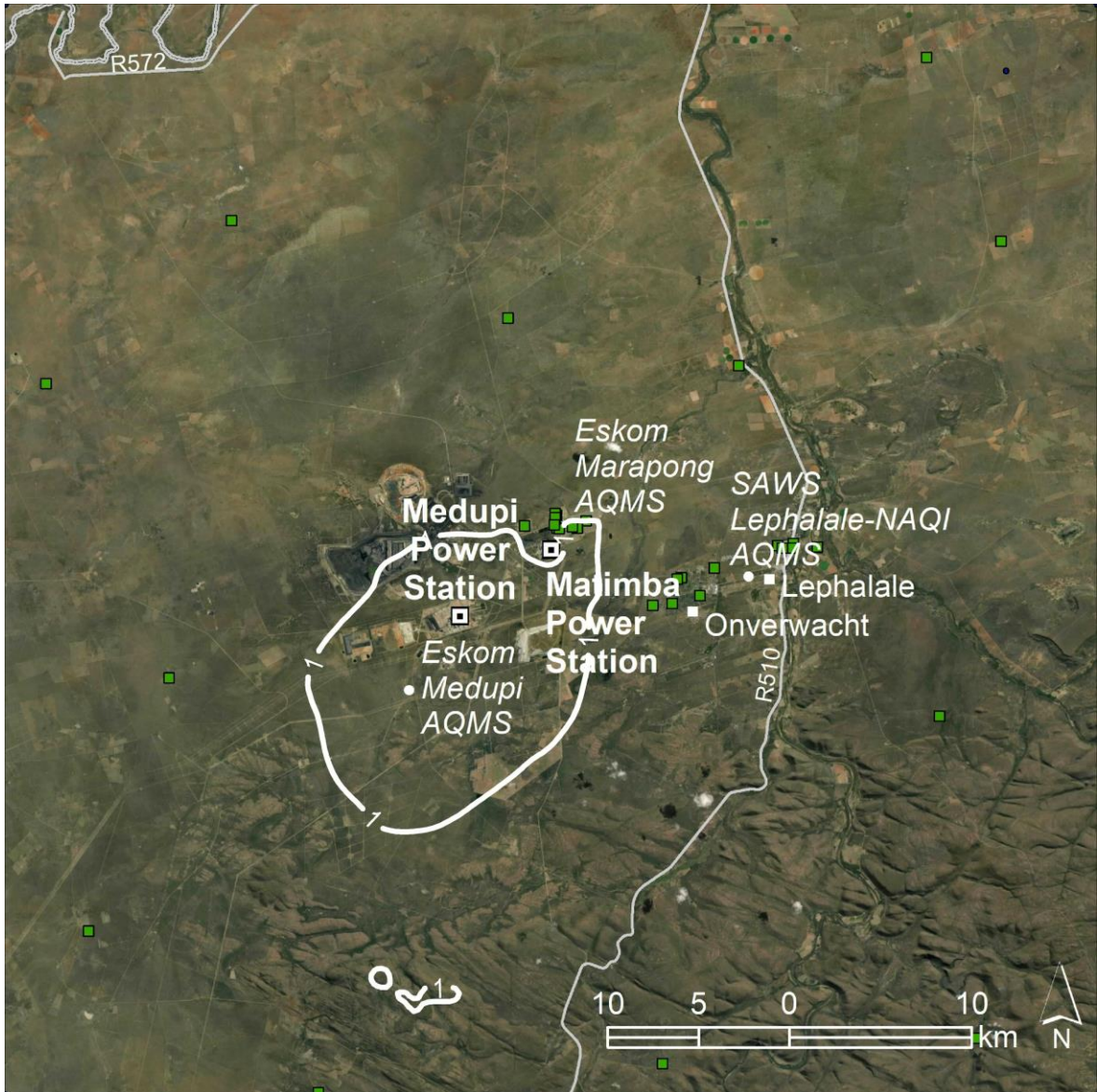
Figure 7-21: Predicted annual average NO 2 concentrations in µg/m 3 resulting from emissions from Matimba: Scenario B (2031) (NAAQS Limit is 40 µg/m 3 )
