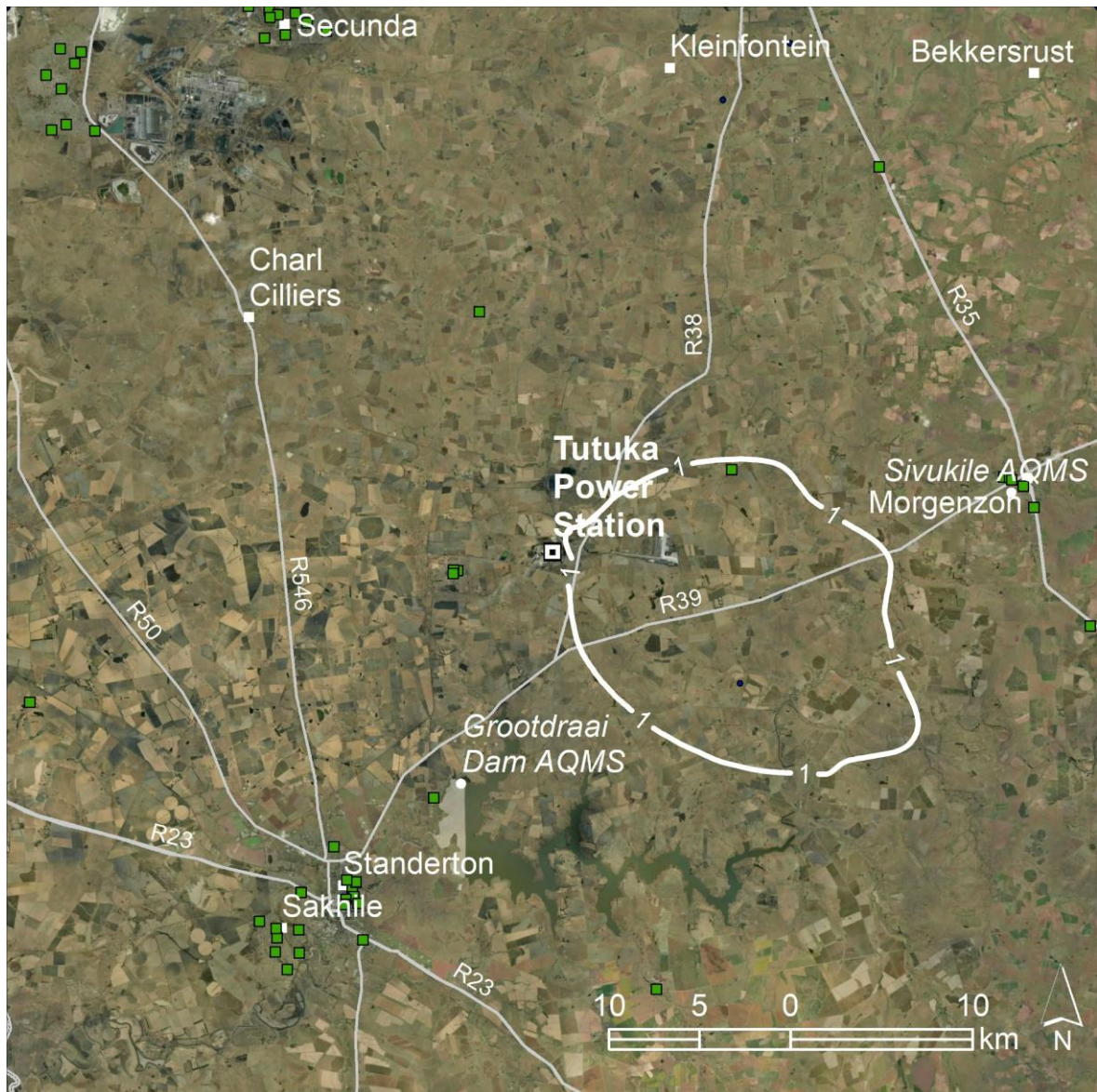
Figure 7-14: Predicted annual average \text{SO}_2 concentrations in \mu\text{g}/\text{m}^3 resulting from emissions from Tutuka: Scenario D (MES) (Current)(NAAQS limit 50 \mu\text{g}/\text{m}^3 )
