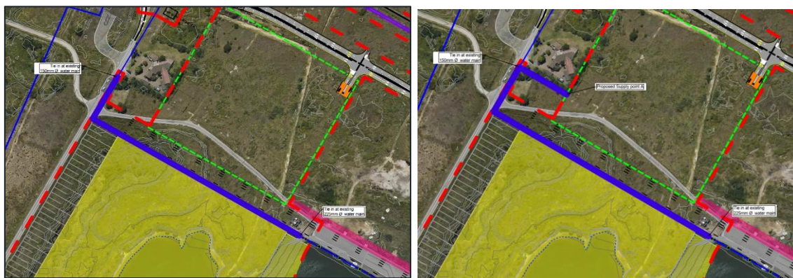
Figure 2-12: Proposed new water main layout (preferred on the left in blue) and proposed supply A (alternative on the right in blue)
