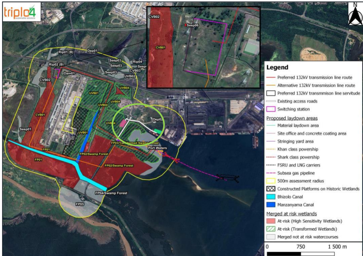
Figure 6-5 – Delineated wetlands for the Gas to Power Project at the PoRB (Triplo4, 2022)
