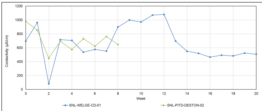
Figure 6-8 - kinetic results showing the evolution of TDS for New Largo Coal residue samples
