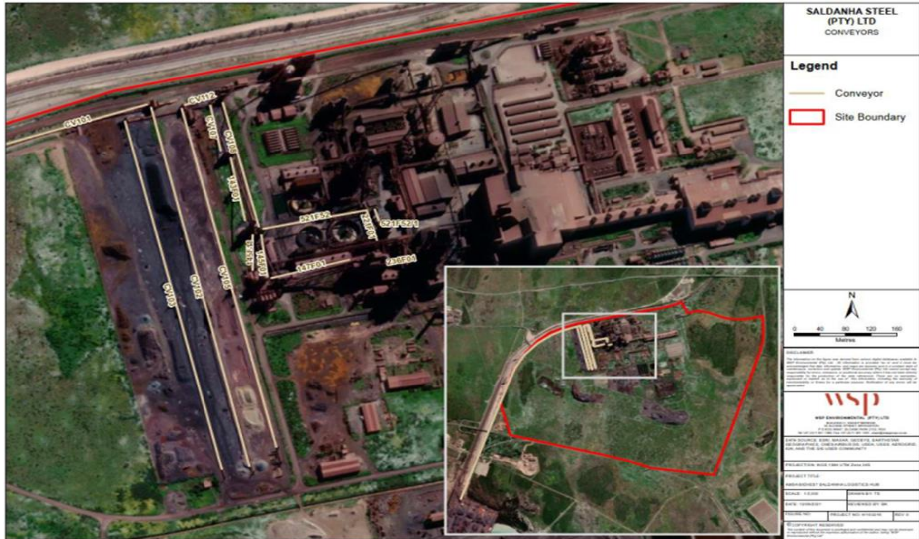
Figure 2-4 - Existing and proposed conveyor system at the Logistics Hub site (WSP, 2023)
