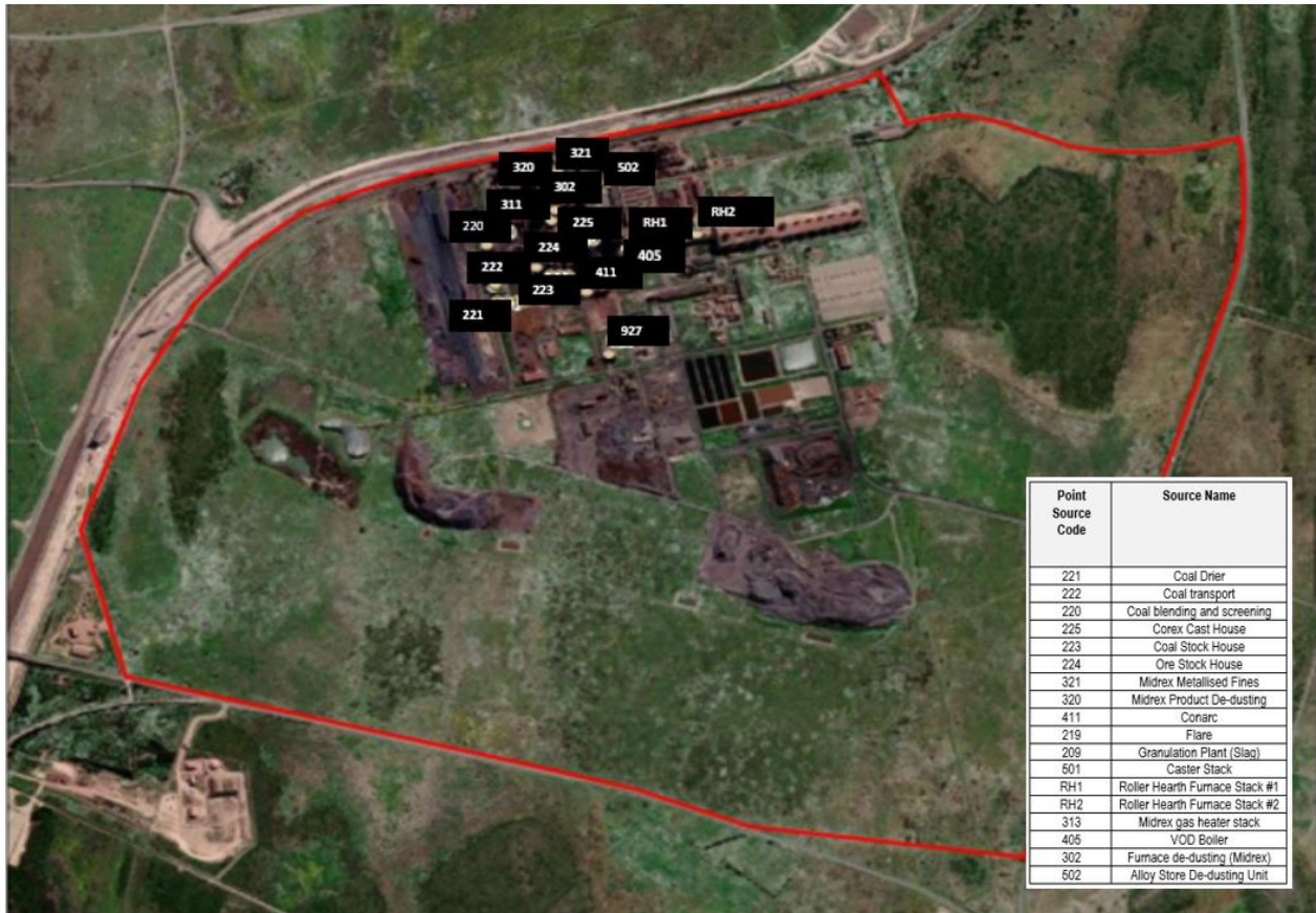
Figure 6-1: Saldanha Steel point source locations
