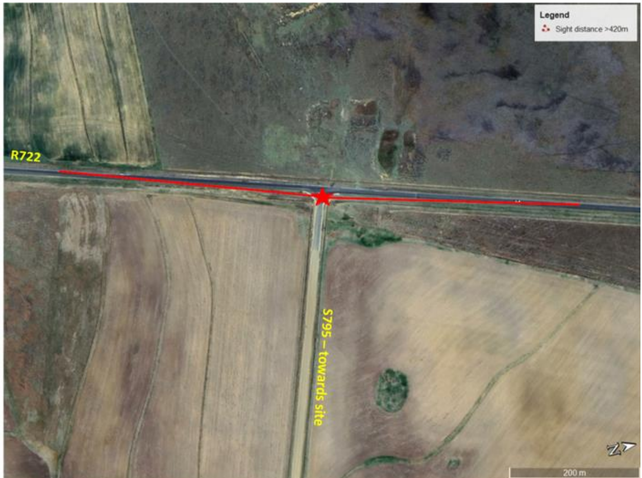
Figure 7-74 - Required Sight distances from S795 onto R722
