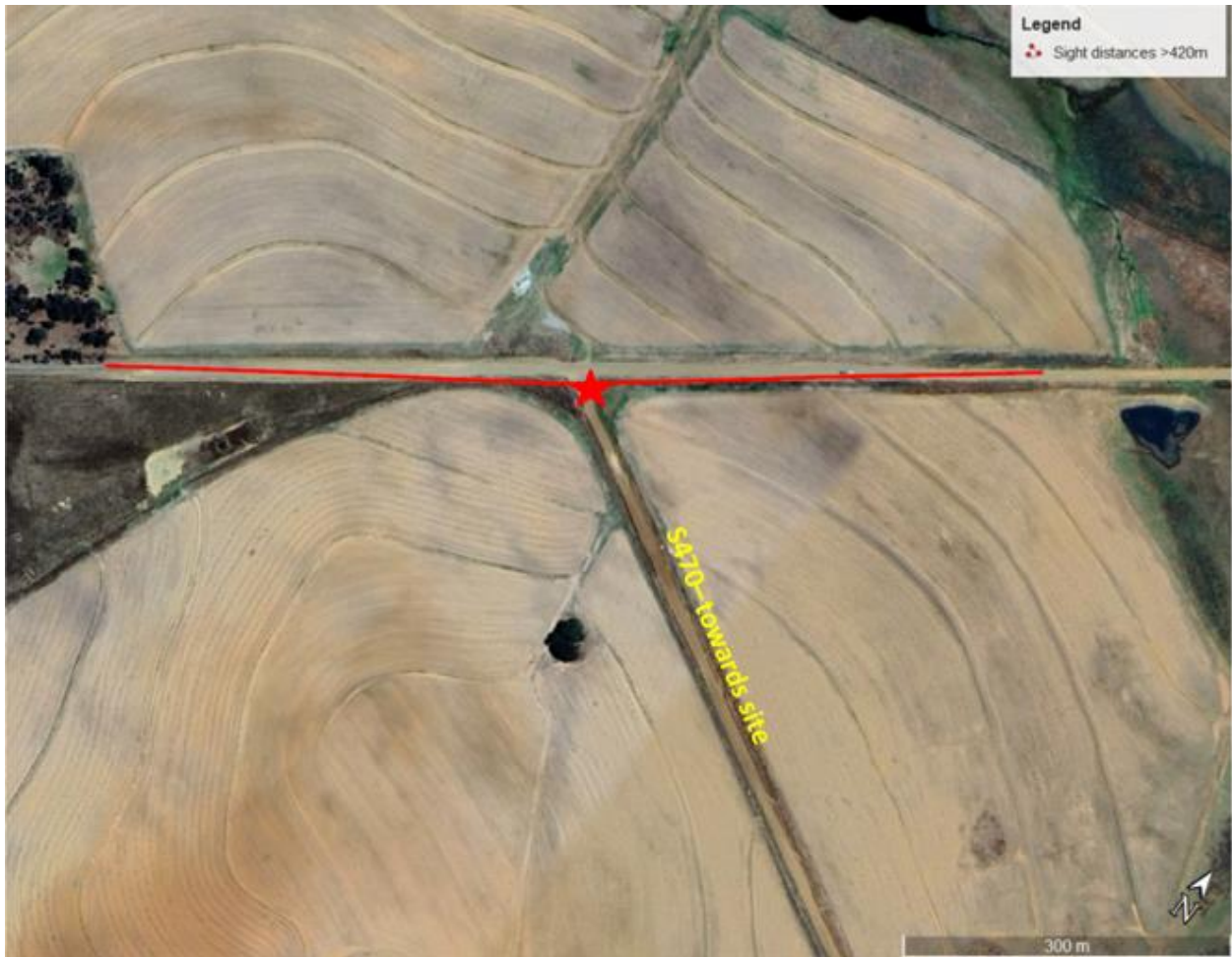
Figure 7-75 - Required Sight distances from S470 onto S722
