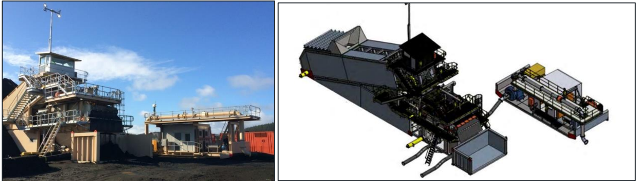
Figure 2-4 - A typical dozer trap mining unit (DTMU) showing the trap on the LHS into which material is dozed and an associated pump unit on the RHS (WSP, 2024a)
