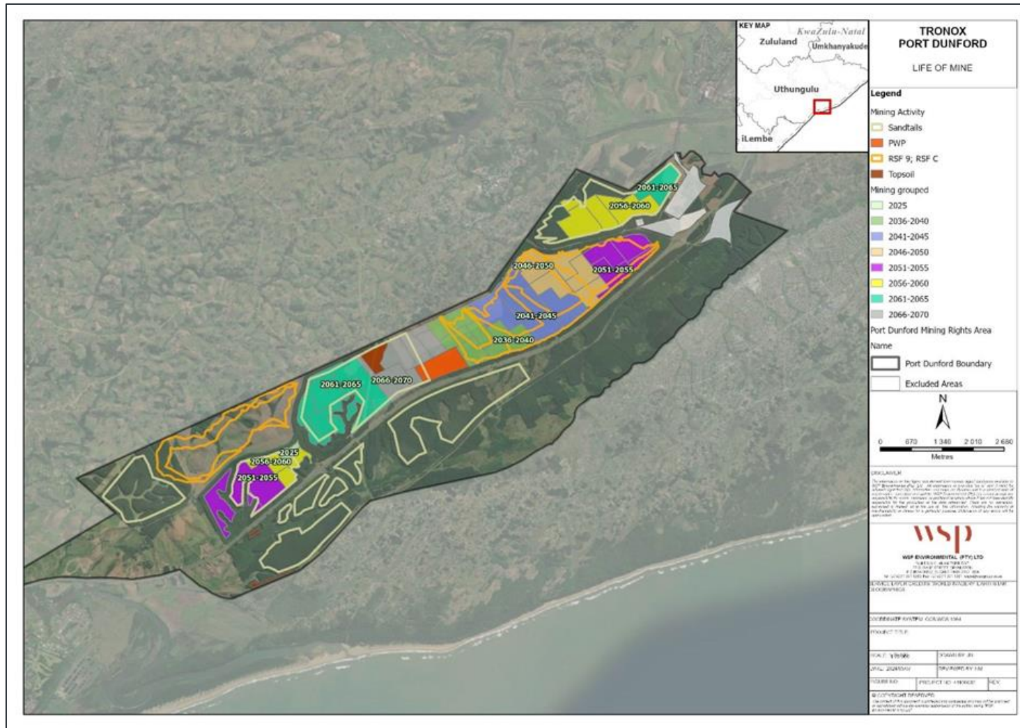
Figure 2-8 - Proposed Phase 2 mining block plan showing 5-year mining windows
