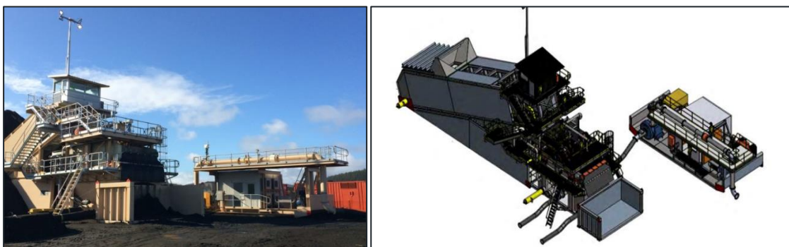
Figure 2-9 - A typical dozer trap mining unit (DTMU) showing the trap on the LHS into which material is dozed and an associated pump unit on the RHS
