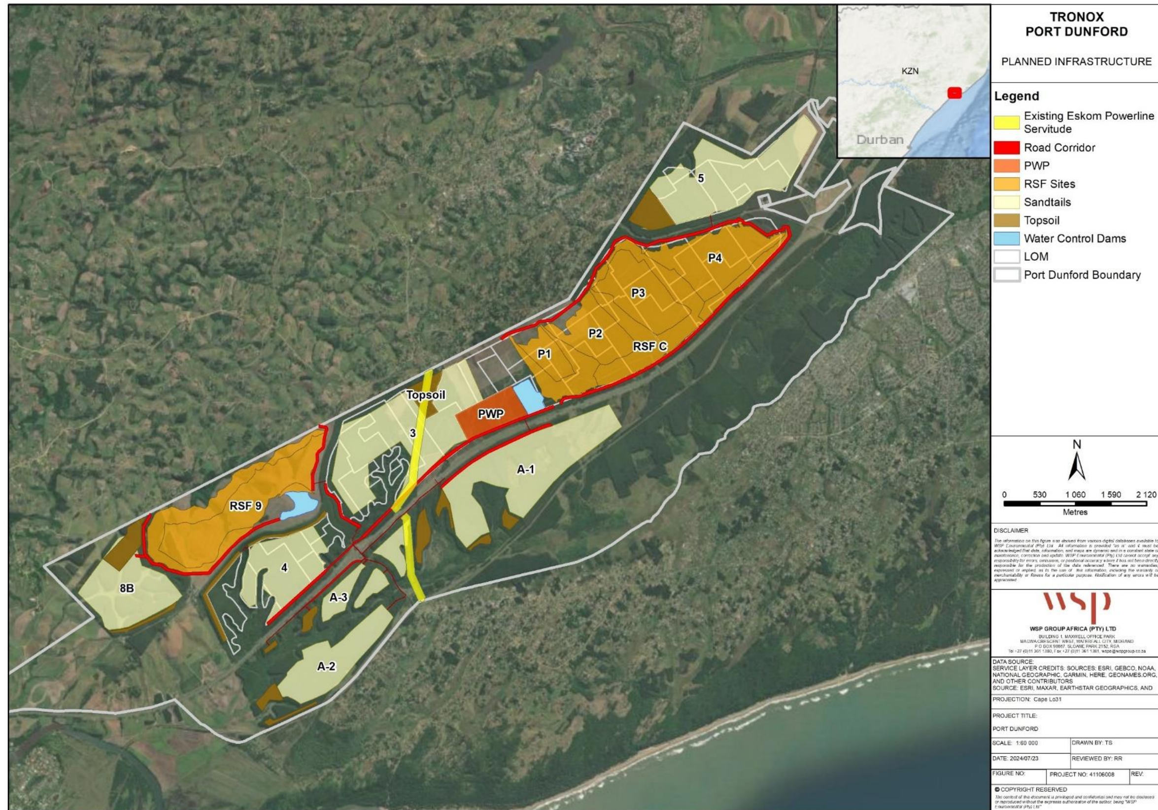
Figure 1-2 - Planned infrastructure for Port Durnford operation
