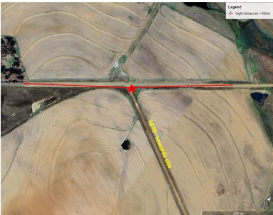
Figure 6-39 - Required Sight distances from S470 onto S722
