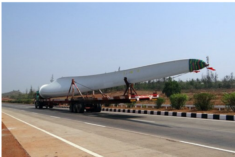
Figure 4-4: Blade transport (Froese, 2019)
