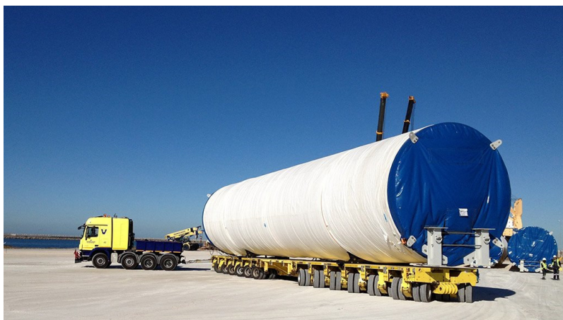
Figure 4-5: Transporting the Tower Sections (Montiea, 2014)
