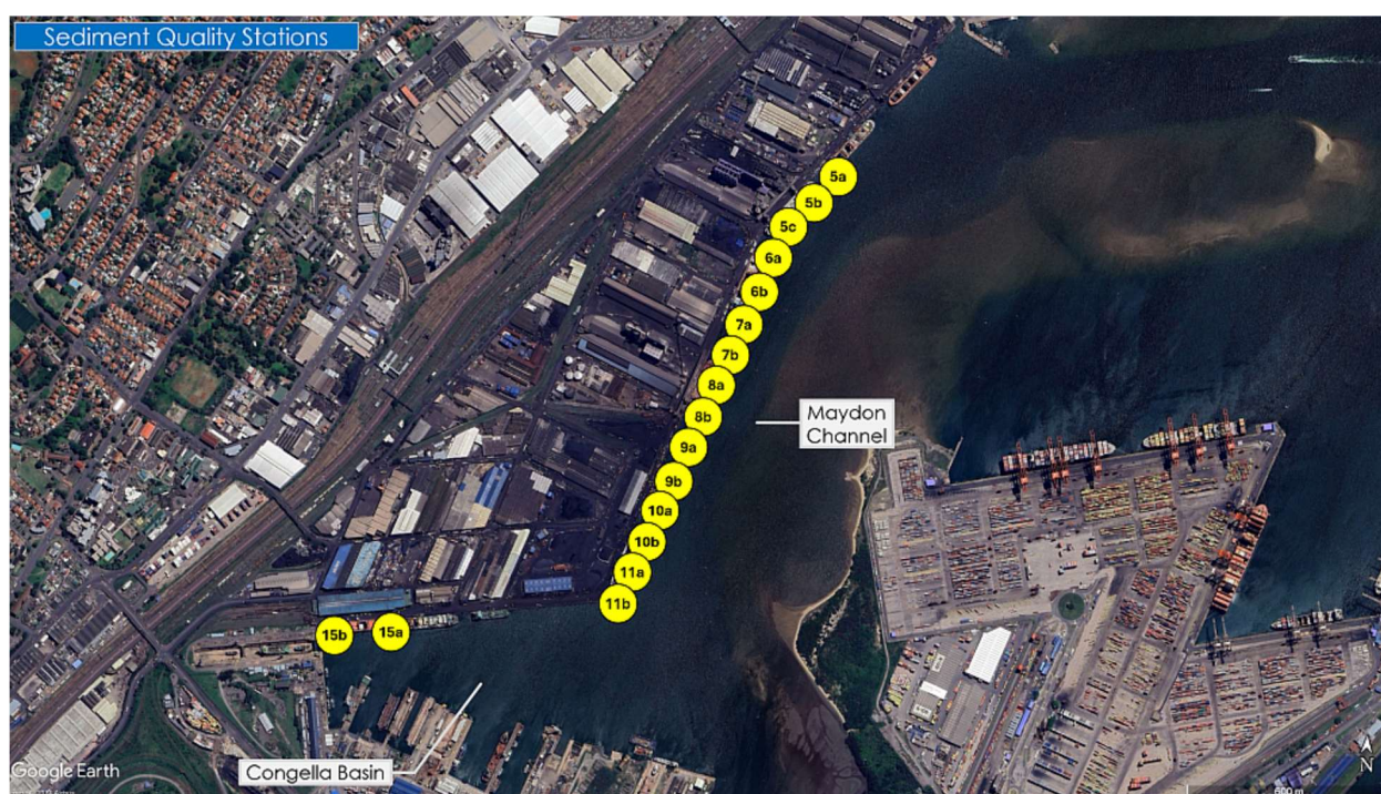
Figure 2. Aerial view of Durban Bay showing the positions (stations) where sediment was sampled in the proposed Maydon Wharf berth deepening dredging footprint for physical and chemical analysis and toxicity testing on May 2024.
