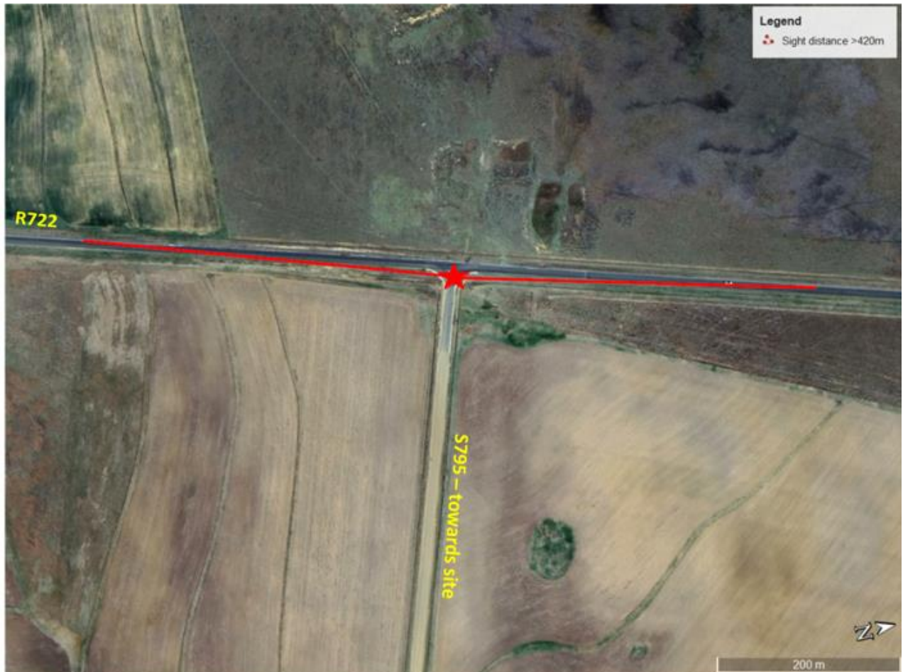
Figure 6-57 - Required Sight distances from S795 onto R722
