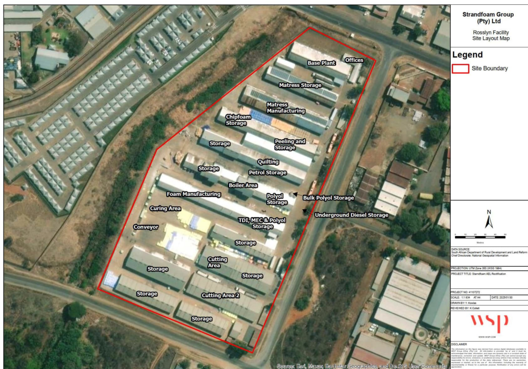
Figure 2-2: Site layout of the Rosslyn Facility
