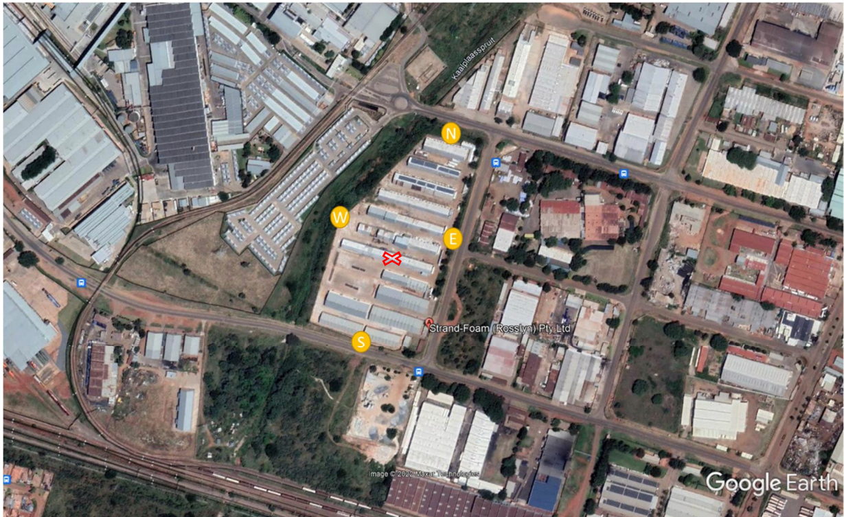
Figure 4: Location of the samplers located just inside the fenceline (North, East, South and West). The location of the Extrusion Line vents is shown approximately with a red cross.
