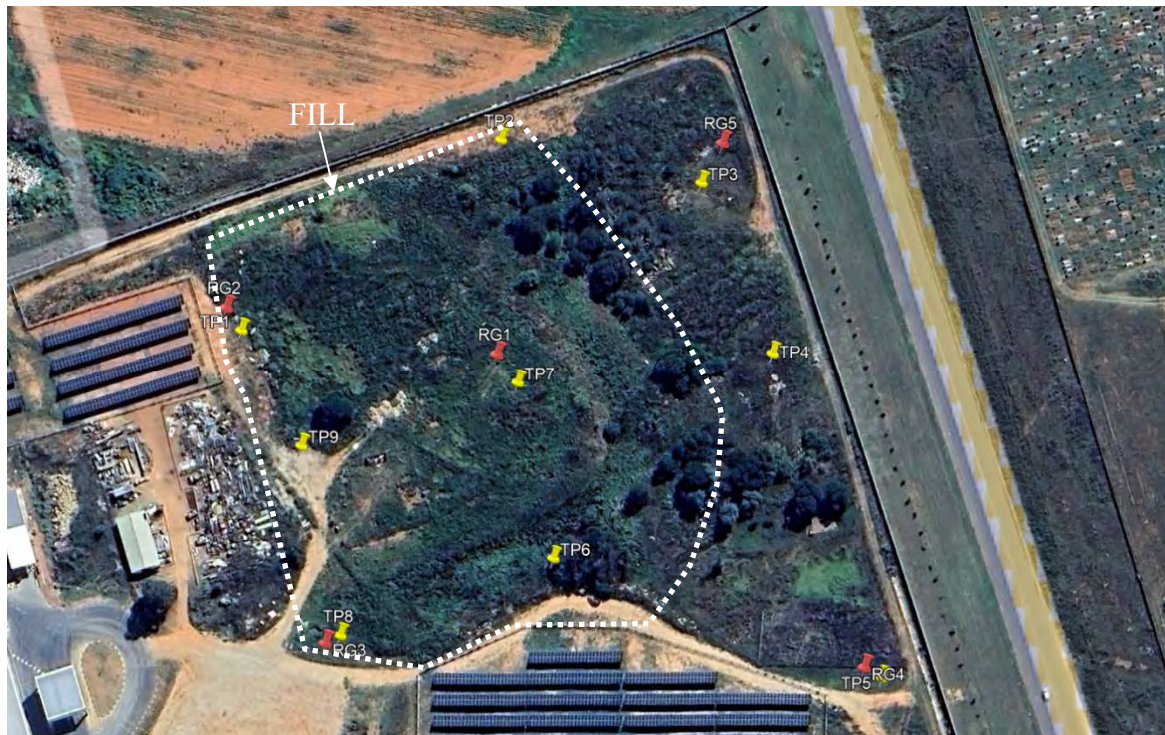
Figure 3-6: Locations of test pits and boreholes
