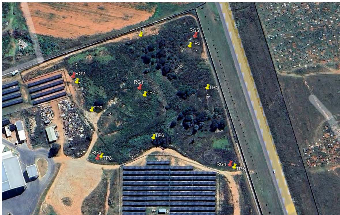
Figure 2-2: Locations of test pits and boreholes
