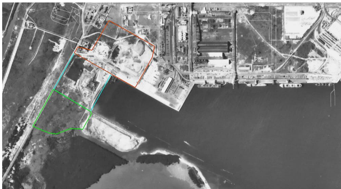
1997 Extensive disturbance associated with the 600 series berth excavation. Note the land reclamation using excavated materials to the south of the berth basin. Similarly, note the mangrove cut line and that the sand barrier has been cut off from land by dredging of the 600 series berth basin
