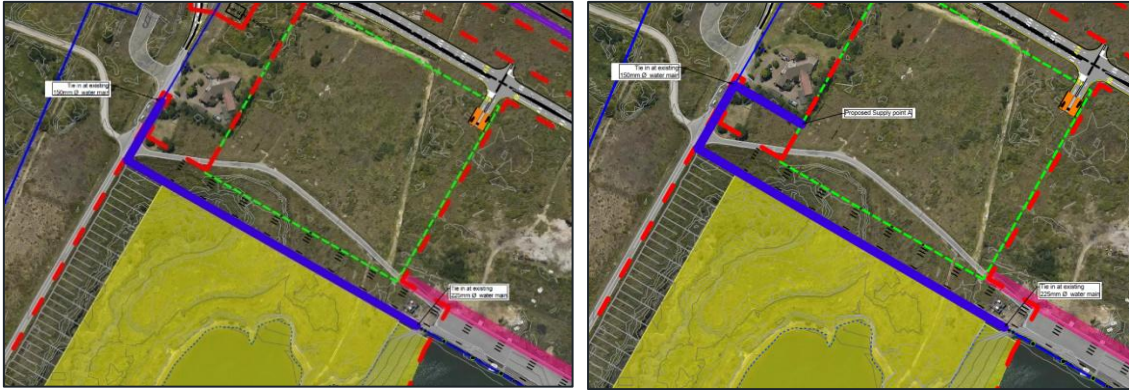
Figure 2-15: Proposed new water main layout (preferred on the left in blue) and proposed supply A (Alternative on the right in blue)
