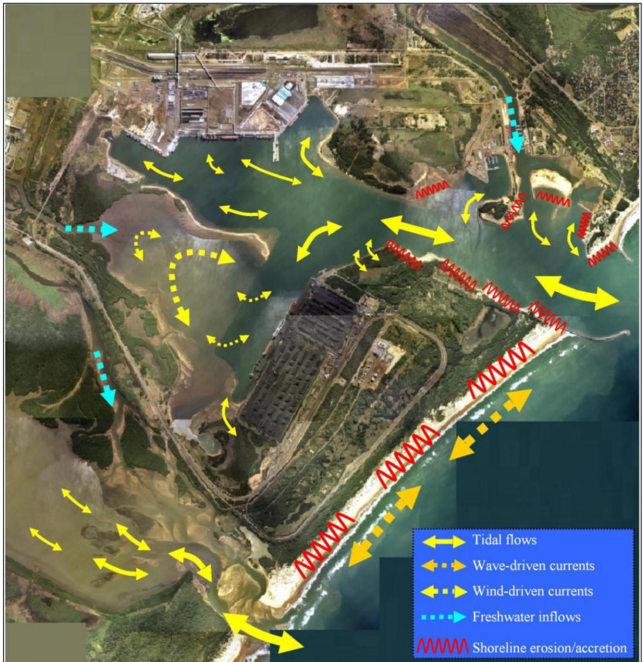
Figure 6-18 - Schematic of the major hydrodynamic processes in the Port of Richards Bay, Mhlathuze Estuary, and shoreline at Richards Bay (from CSIR, 2005)
