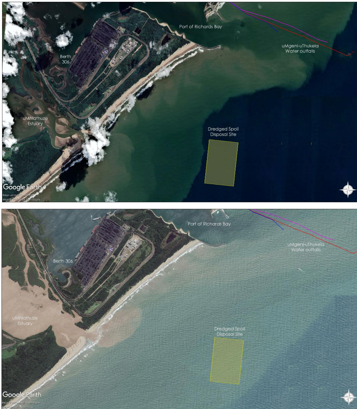
Figure 6-12 - Sediment plumes in the nearshore environment with evidence (lower panel) of naturally elevated turbidity in the surface waters extending as far as the offshore disposal site (CSIR, 2025).
