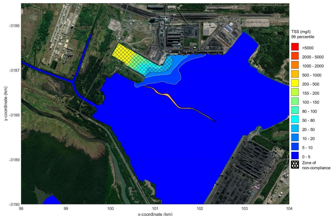
Figure 6-16 – 99 th percentile exceedance contours of TSS concentration in bottom waters within the port, indicating the zone of non-compliance with a 20 mg/ℓ threshold.
