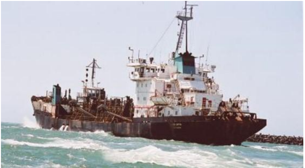
Figure 2-3 - The Ingwenya , the hopper dredger operated at Richards Bay by Transnet NPA Dredging Services.
