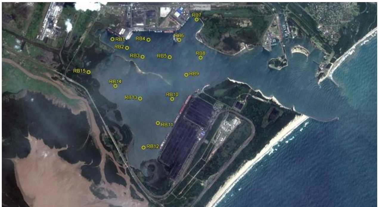
Figure 4-14 - Map of Richards Bay showing the positions where in situ water quality measurements (i.e., temperature profiles) were made for the Richards Bay Capacity Expansion EIA.
