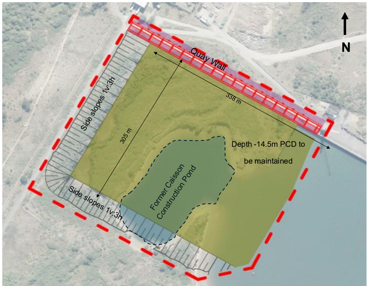
Figure 2-1 - Basin area to be excavated plus outline of the existing pond where caissons were formerly cast (Source WSP, 2024b).
