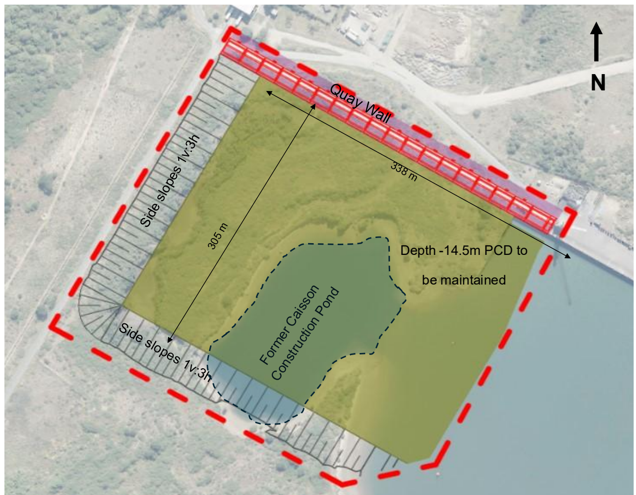
Basin area to be excavated plus outline of the existing pond where caissons were formerly cast
