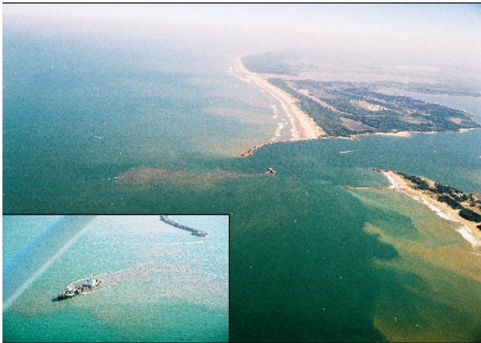
Figure 6-11 – Elevated water column turbidity due to dredging activities at the port entrance and re-suspension of sediments in the nearshore environment (Photo courtesy of Mr C.J. Ward as reported in Weerts, 2008).
