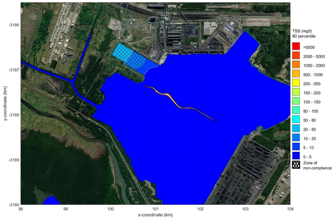
Figure 6-2 - 80 th percentile exceedance contours of the elevation in TSS concentration in surface waters within the port.
