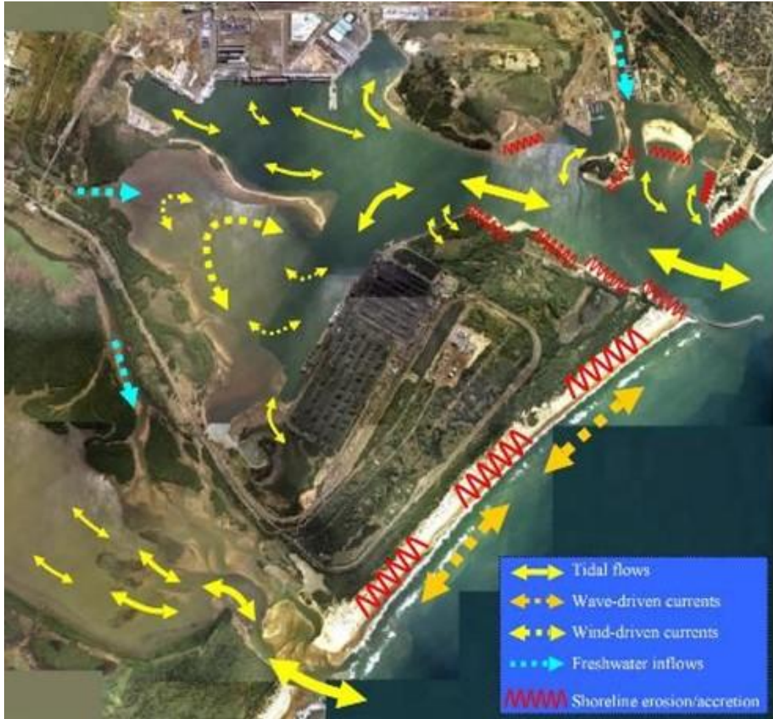
Figure 4-25 - Schematic of the major hydrodynamic processes (Source: (CSIR, 2005a)).
