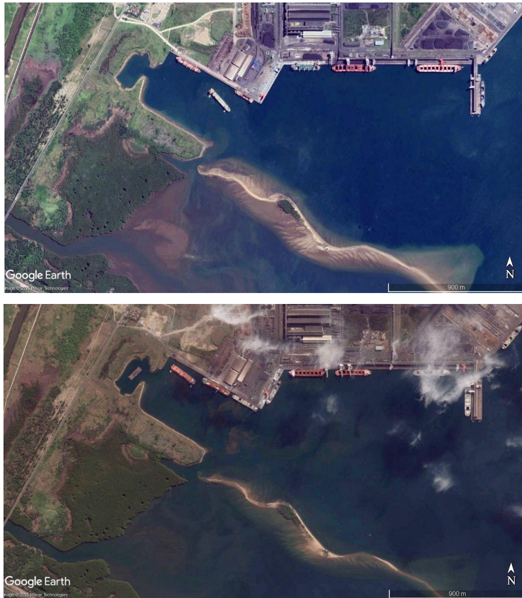
Figure 6-4 - Sediments driven into suspension by ship berthing activities in the 600 series basin on 27 March 2016 (upper panel) and 9 August 2016 (lower panel) in the Port of Richards Bay (Source: GoogleEarth).
