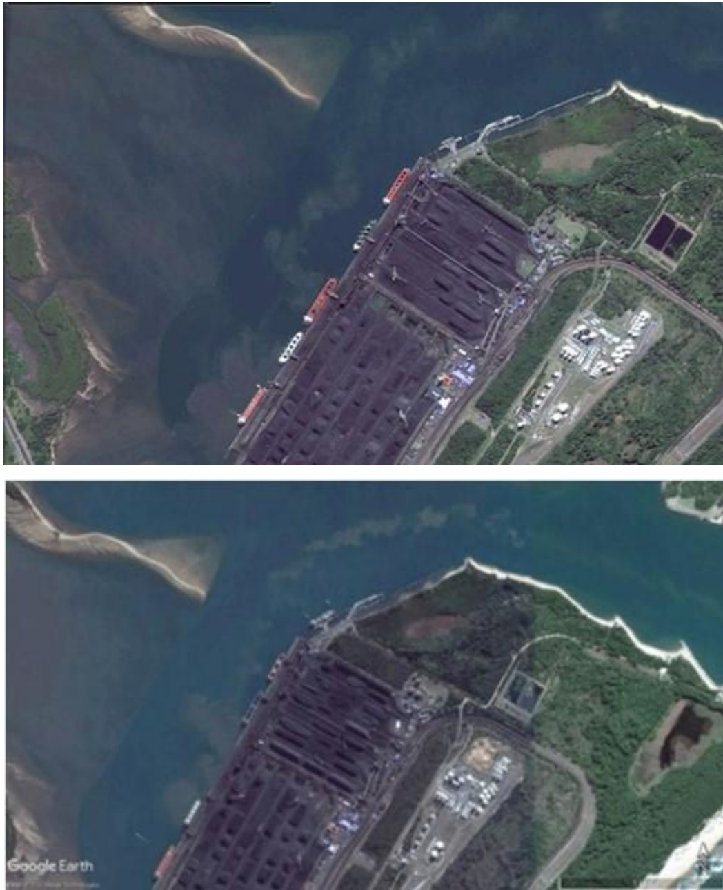
Figure 6-6 - Sediment driven into suspension by ship berthing activities in the coal basin in the Port of Richards Bay on 3 May 2014 (upper panel) and in the coal basin and entrance channel the Port of Richards Bay on 29 July 2015 (lower panel). (Source:GoogleEarth)
