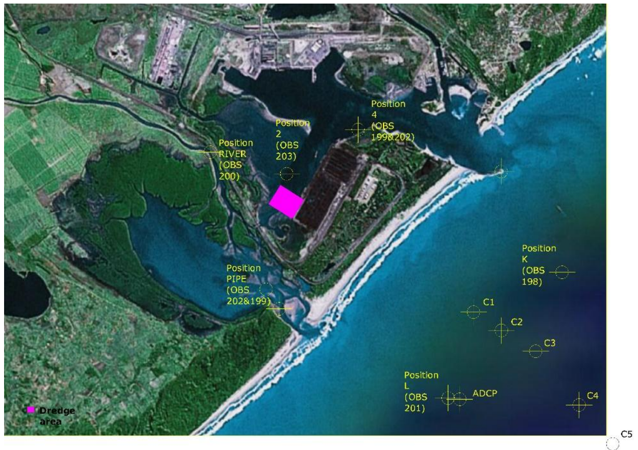
Figure 4-36 - Locations of the OBS moorings K and L during the Berth 306 Dredge monitoring programme
