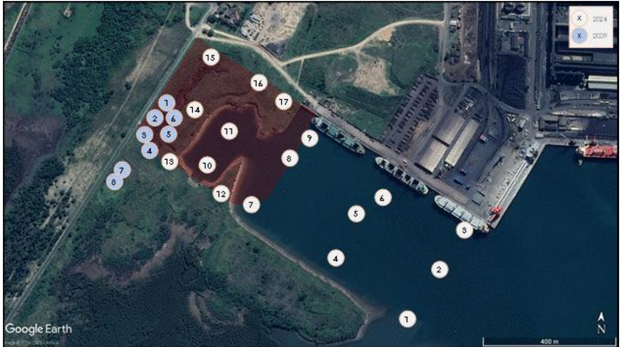
Figure 2-2 - Aerial views of the Port of Richards Bay, showing the positions where sediment and soil was sampled in and near the 600 Berth Basin in November 2024 and where soil was sampled in 2009 (CSIR, unpublished data). The red shaded area denotes the proposed Berth 605 dredging and excavation footprint (Source: CSIR, 2024)
