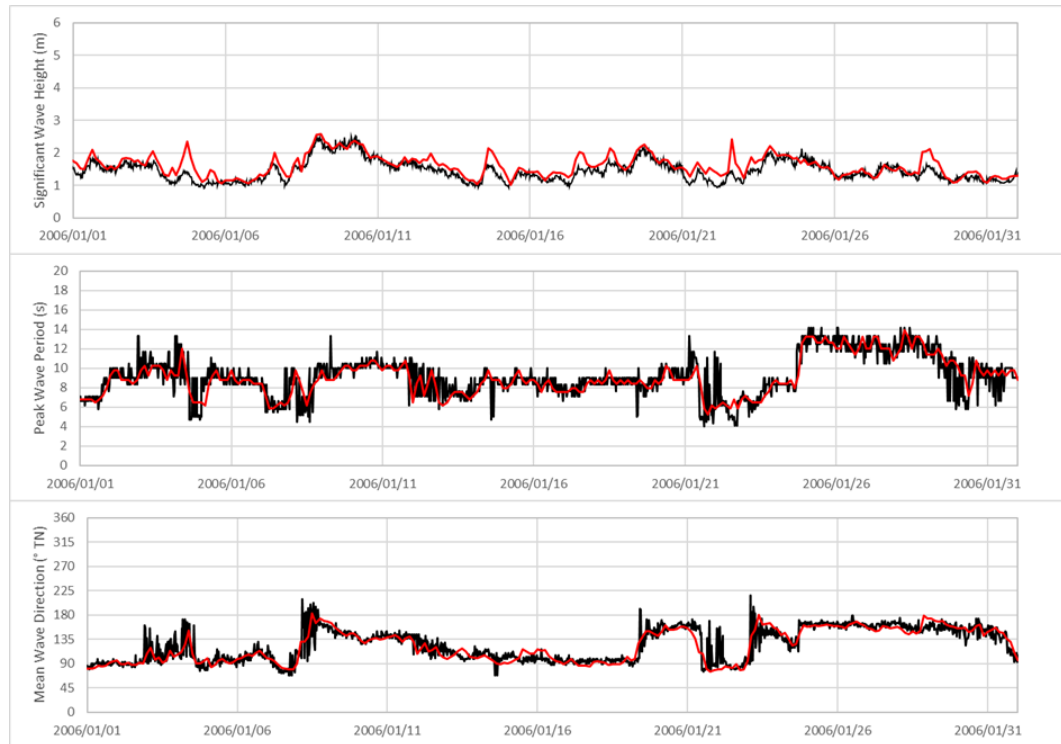
Figure 5-10 – Measured (black) and modelled (red) wave parameters at Waverider buoy during January 2006.
