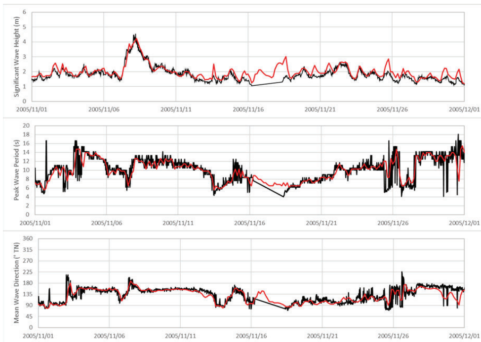
Figure 5-8: Measured (black) and modelled (red) wave parameters at Waverider buoy during November 2005
