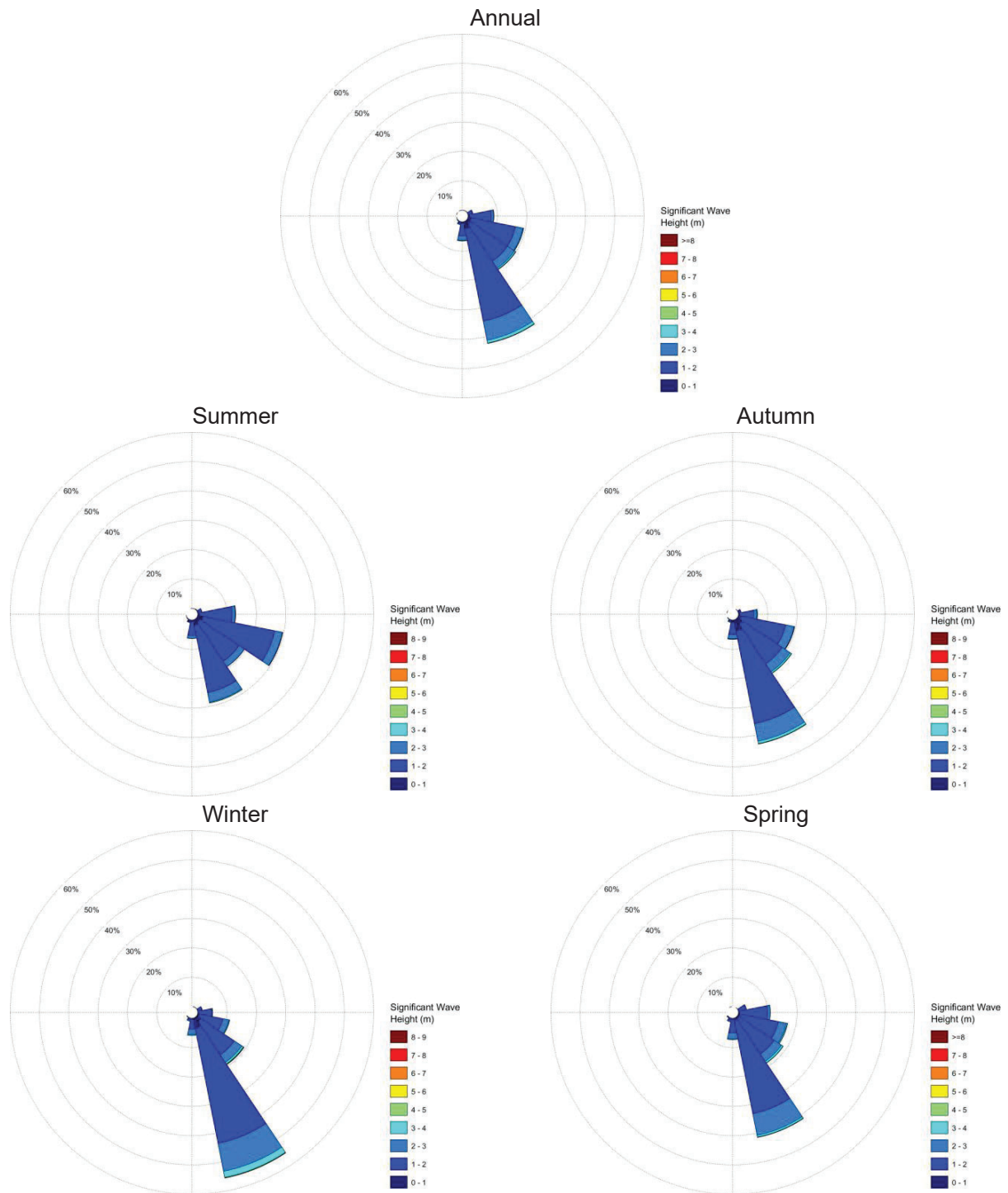
Figure 3-4: Wave roses based on Waverider data collected outside Port of Richards Bay, (Latitude: -28.8265°S, Longitude: 32.1040 °E) for the period of 1979 to 2002.
