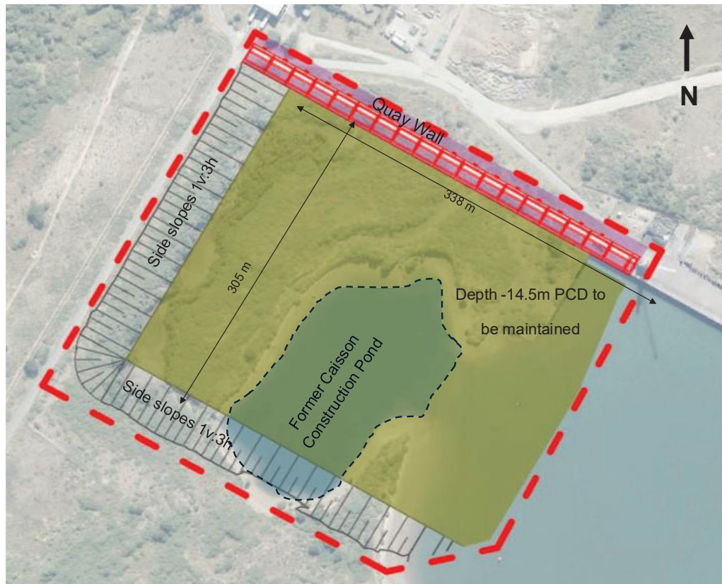
Figure 2-1: Basin area to be excavated plus outline of the existing pond where caissons were formerly cast (Source WSP, 2024b).
