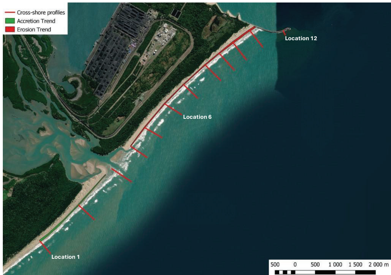
Figure 7-3: Erosion and Accretion zones resulting from dredge disposal activity
