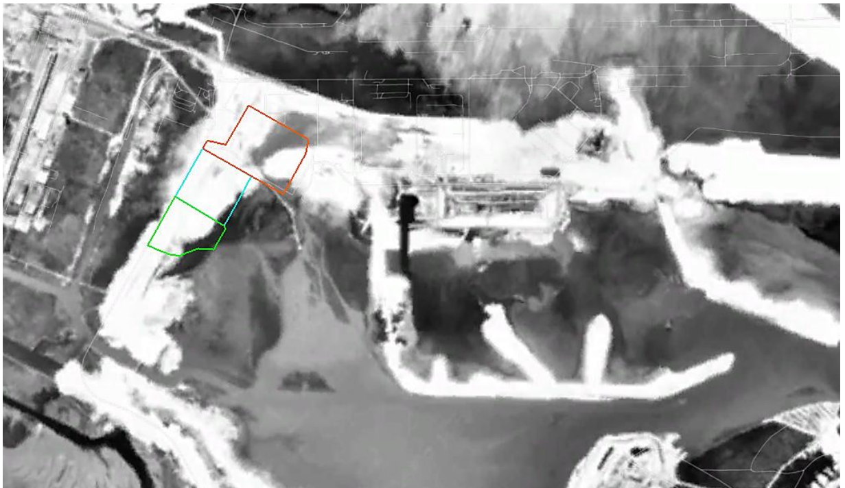
1975 The project and compensation areas in relation to initial sand backfill and stabilisation as part of early port development earthworks. Note the redirected river mouth south of Harbour road and the development of a sand barrier north of which the initial Port basin was deepened.
