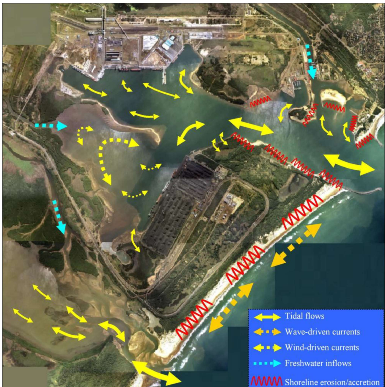
Figure 18. Schematic of the major hydrodynamic processes in the Port of Richards Bay, Mhlathuze Estuary, and shoreline at Richards Bay (from CSIR, 2005).
