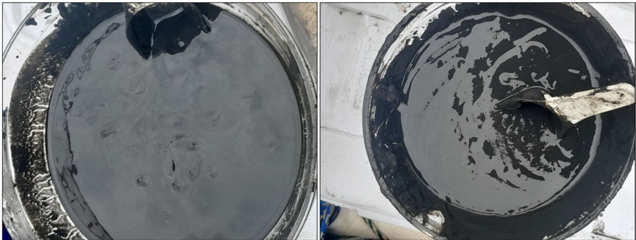
Figure 27 Sediment sampled at Station 6 (left) and Station 9 (right) in the 600 Berth Basin in the Port of Richards Bay by the CSIR in November 2024. Note the dark colour of the sediment, presumably imparted by coal particles.
