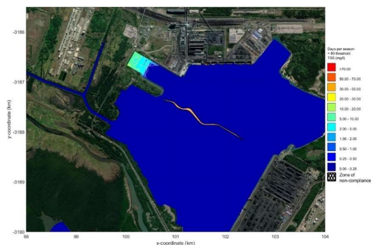
Figure 101. Days of exceedance contours of suspended sediment threshold of 80 mg.L -1 in surface waters within the Port of Richards Bay (van Ballegooyen et al. , 2025).
