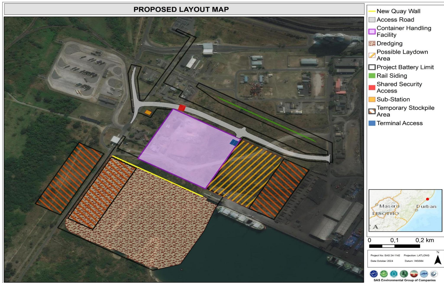
Figure 3: Proposed layout of the Berth 605 at the Port of Richards Bay.
