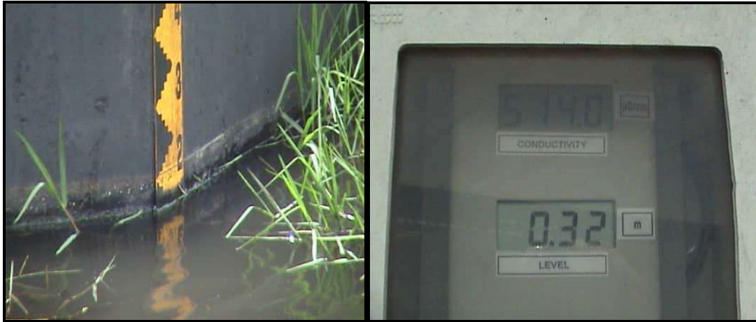
Figure 4 Weir gauge plate as well as the electronic display for depth and conductivity
