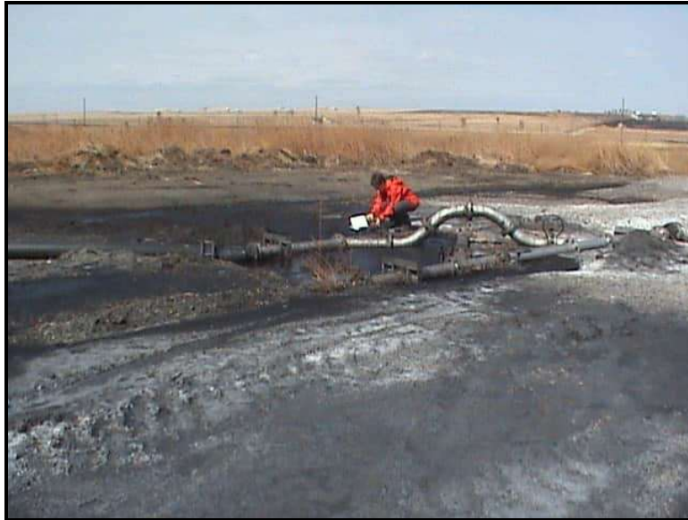
Figure 31 Photograph of leaking valve below Twistdraai Export plant discard dump
